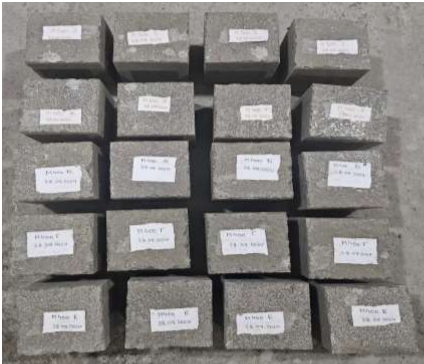
Picture 3. 10x10x10 samples of B30(M400) class concrete
