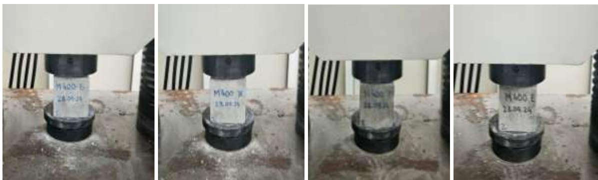
Picture 4. Testing the compressive strength of B30 (M400) class concrete in a hydraulic press
