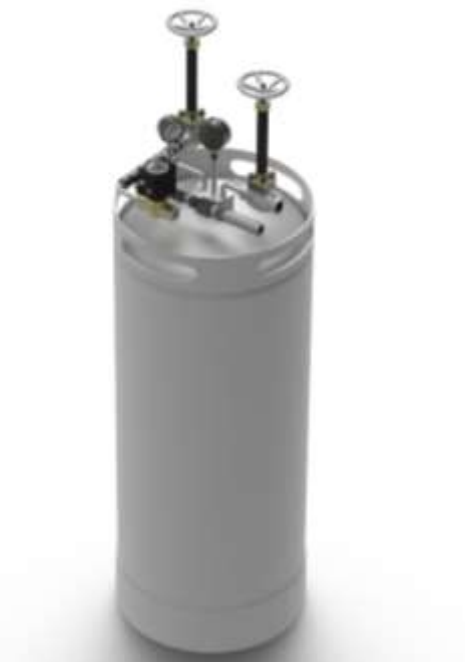
Figure 2. Liquid Hydrogen Tank 3D Design.
